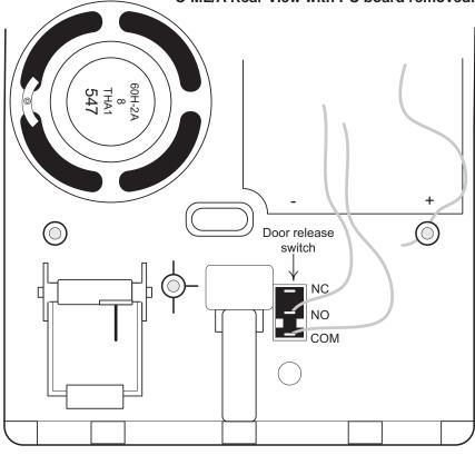
C-ML/A Rear View with PC board removed.
